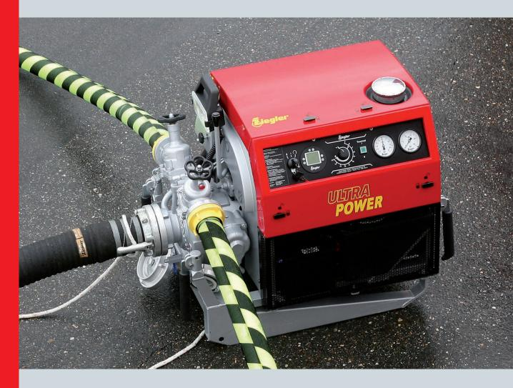
Portable pump with Volkswagen BVS 4-stroke Otto engine, electronic injection, designed as PFPN 10-1000 und 10-1500, tested in compliance with DIN EN 14466.
