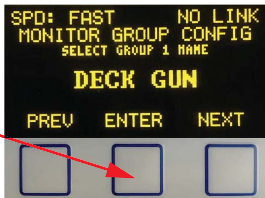
Figure 5.4d Group Control Configuration Step 4
